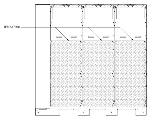
Figure 9-2. UPM Section Air Filter Locations
